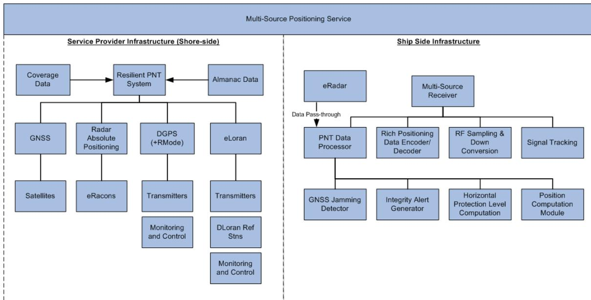
**Figure 3.1 – Top down design of Multi-Source Positioning Service. (Note that radar absolute positioning, although demonstrated, will not be implemented within the timeframe of ACCSEAS).**
