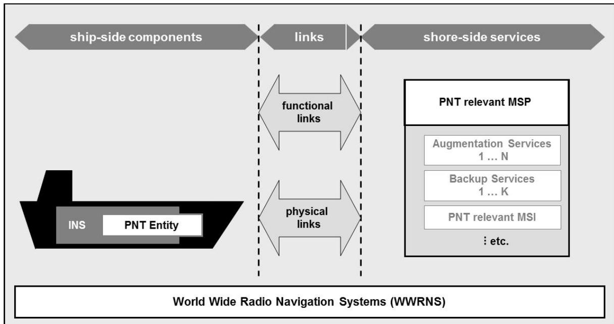
**Figure 2.1 - Generic architecture of the maritime Integrated PNT system. After [1].**
