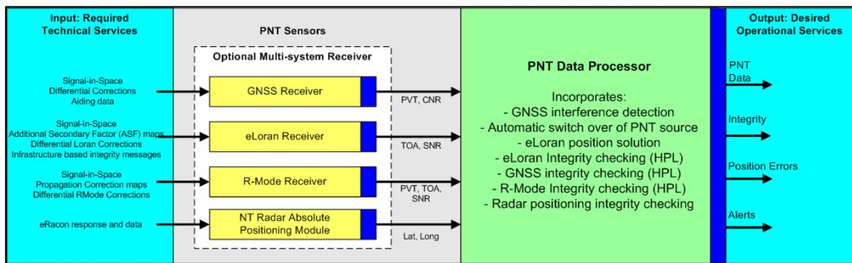
**Figure 2.3 – Structure of the ACCSEAS ship-side Multi Source Positioning Service architecture.**
